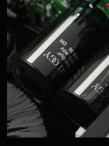
inertia of the heatsink, keeps the devices in their optimum operating condition and improves sound quality. Feeding the 925 is a substantial faraday screened power supply transformer with separate windings and rectifiers for either channel. Custom Trilogy reservoir capacitors smooth each channel of the output stage DC and valve HT supplies.
