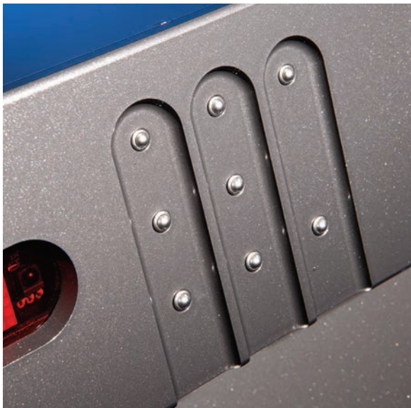
ABOVE: Input selection and menu selection entries are made via these ball-bearing push buttons on the 909
