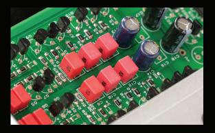
The high bandwidth and low distortion topology uses active current sources and cascode gain blocks with zero global feedback.
